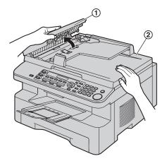
3 Clean the document feeder rollers (③) with a cloth moistened with isopropyl rubbing alcohol, and let all parts dry thoroughly.
